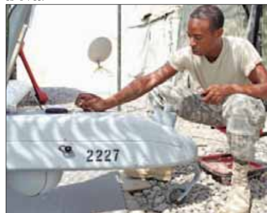
Army Sgt. Christopher Johnson, Bravo Company, 173rd Special Troops Battalion (Airborne) takes the screws out of the nose of a RQ-7 Shadow 200 Unmanned Aerial Vehicle June 19 during "preventive maintenance daily" on Forward Operating Base Fenty in Jalalabad, Afghanistan.
